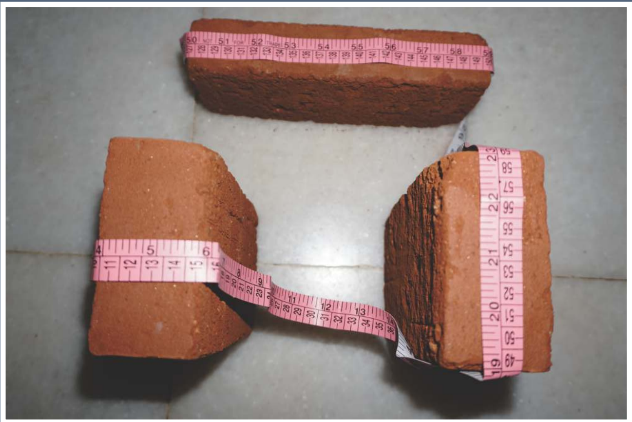
Picture of the bricks with measurements
